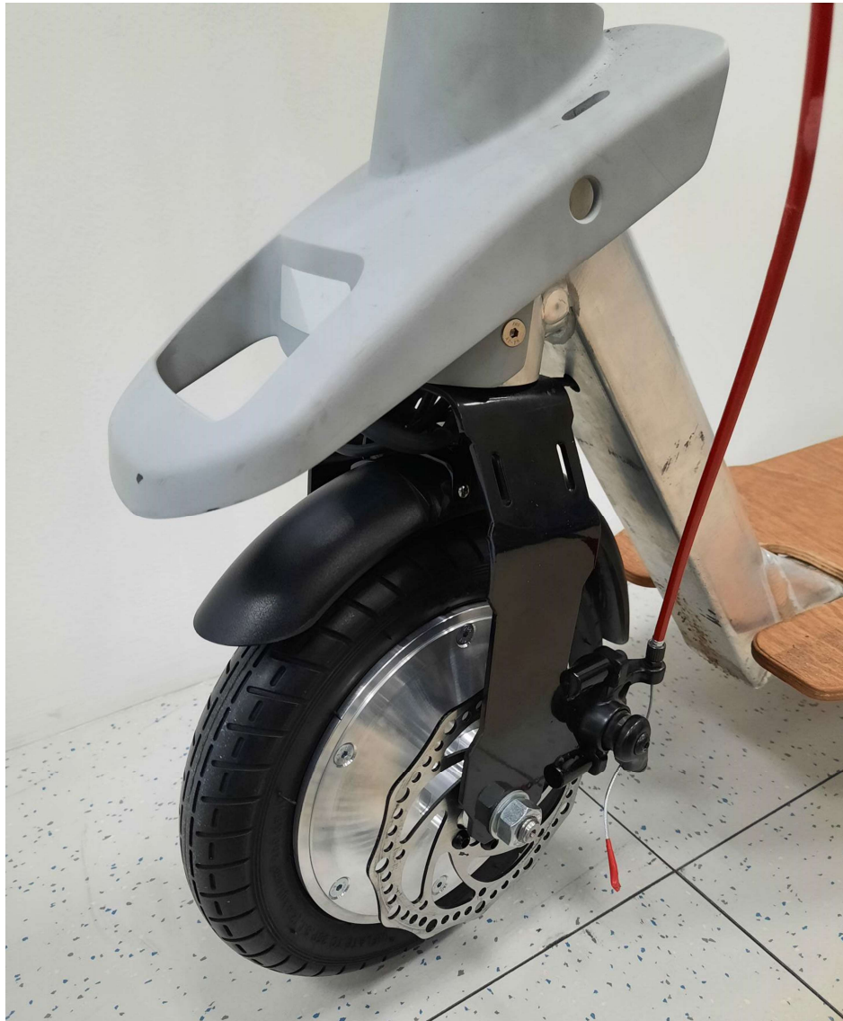
Figure 5: HUB motor integrated in e-kick scooter.
