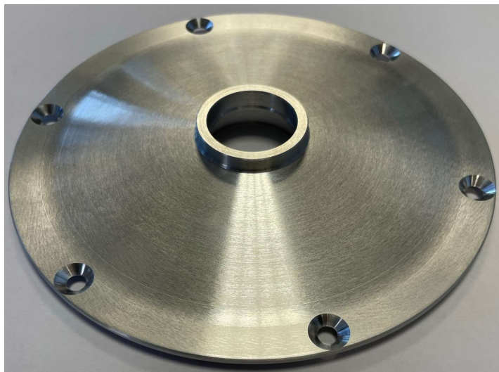
Figure 3: HUB motor cover B.
