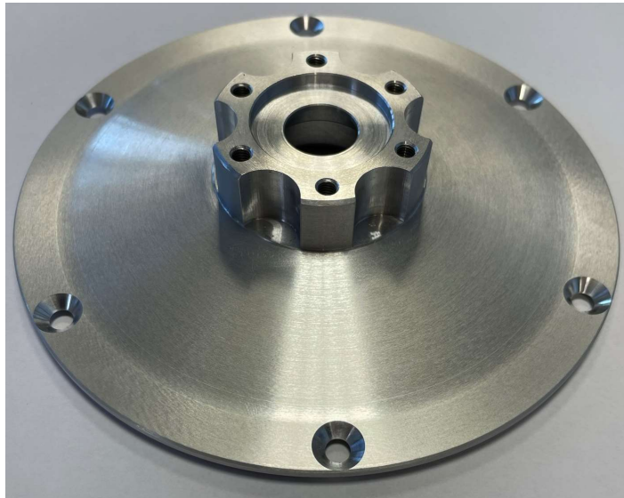
Figure 2: HUB motor – side cover A.
