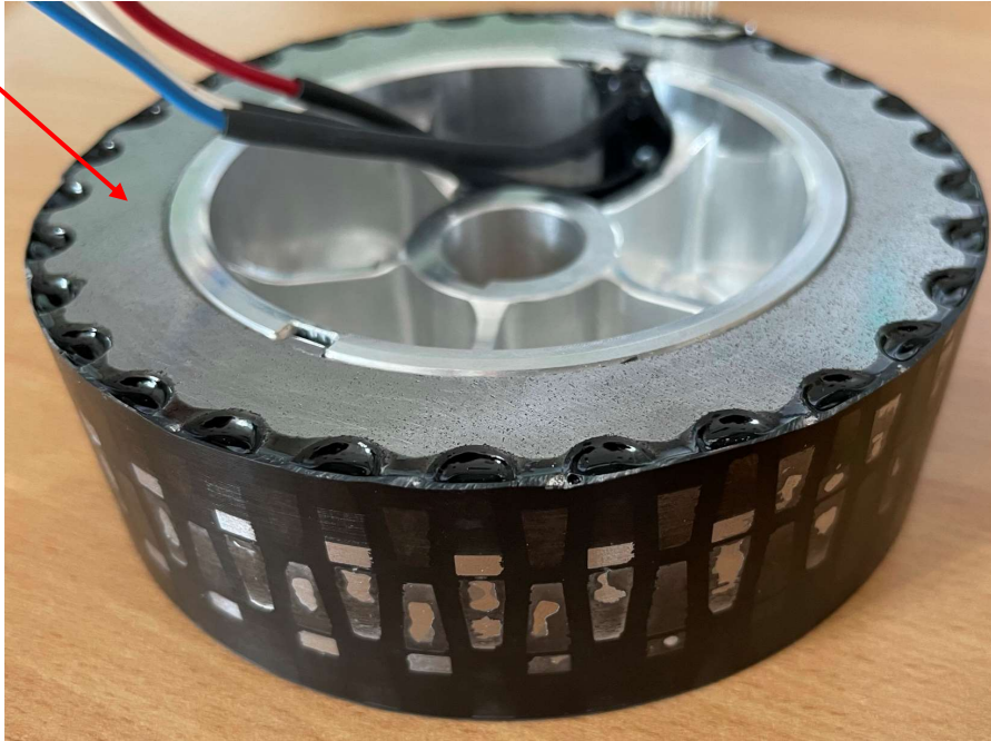
Figure 6: TFM stator – potted.
