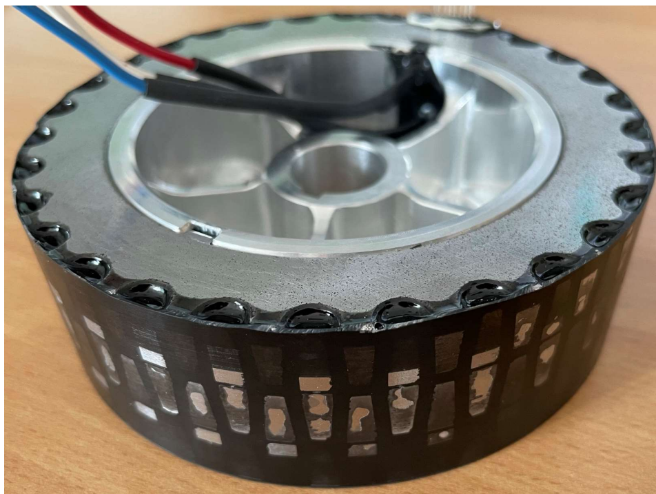
Figure 12: Potted stator stack.
