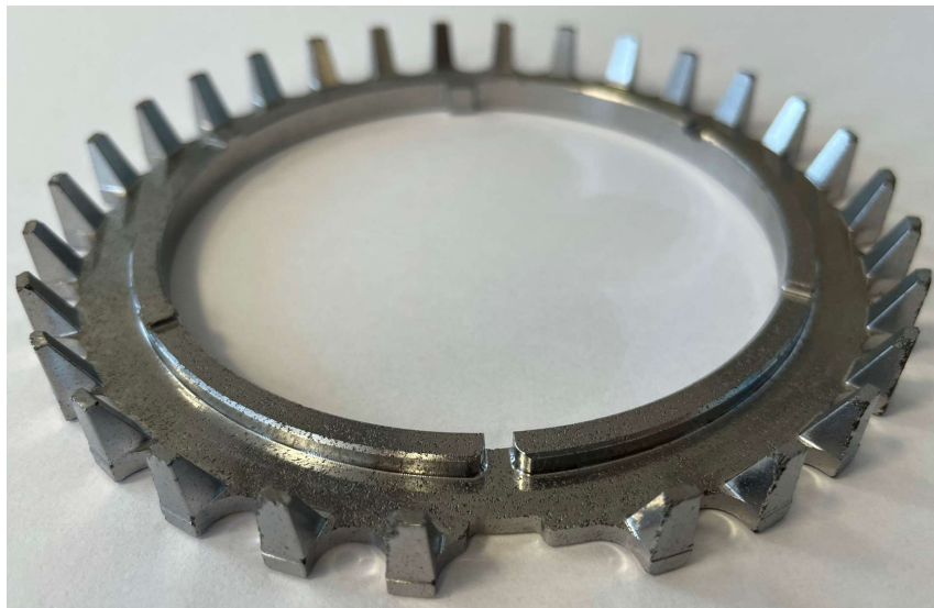
Figure 10: Machined motor phase halve.
