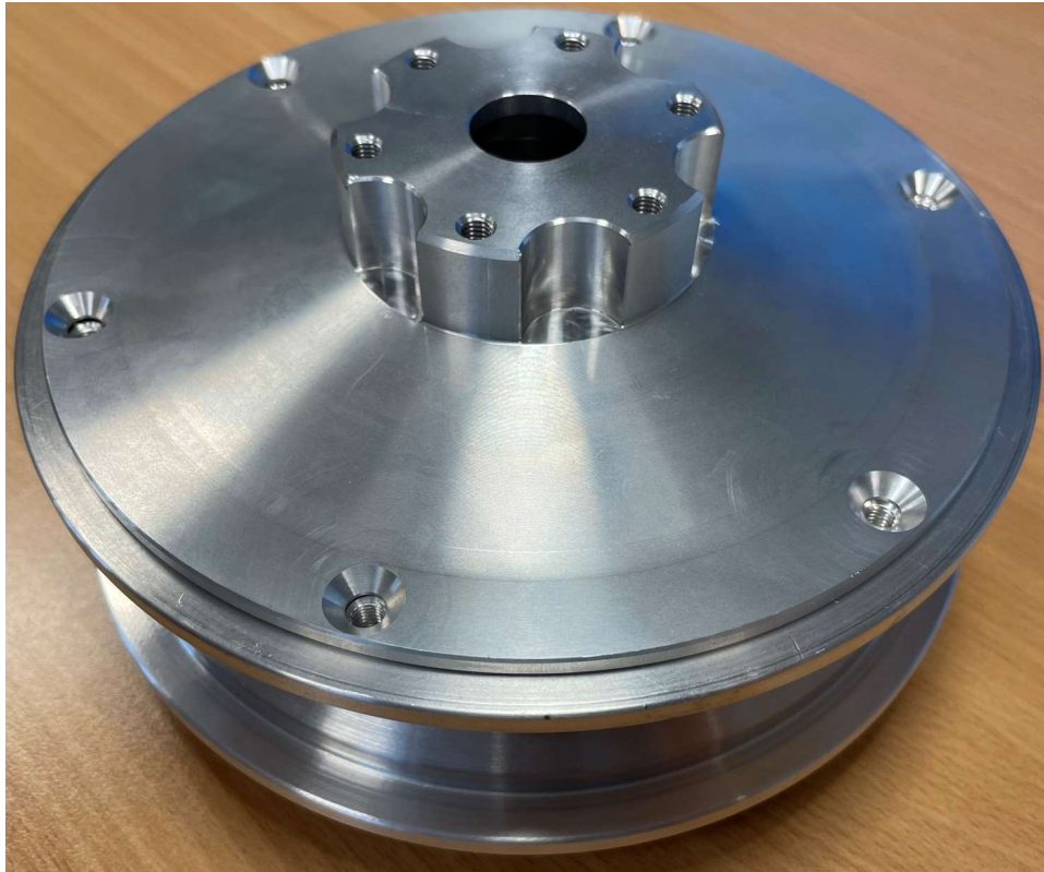
Figure 13: Motor housing assembly.
