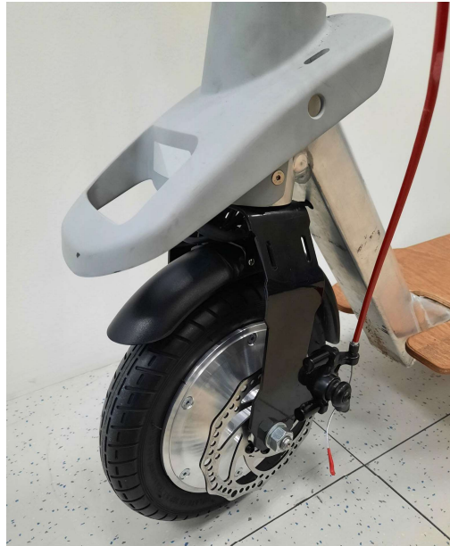
Fig. 7 HUB motor integrated in e-kick scooter.
