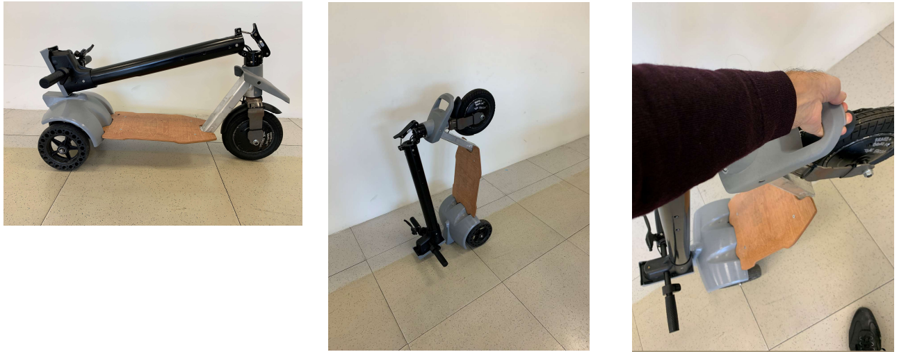
Fig 5 - DREEM scooter 1 st design – foldability solution “suitcase-like” experience
